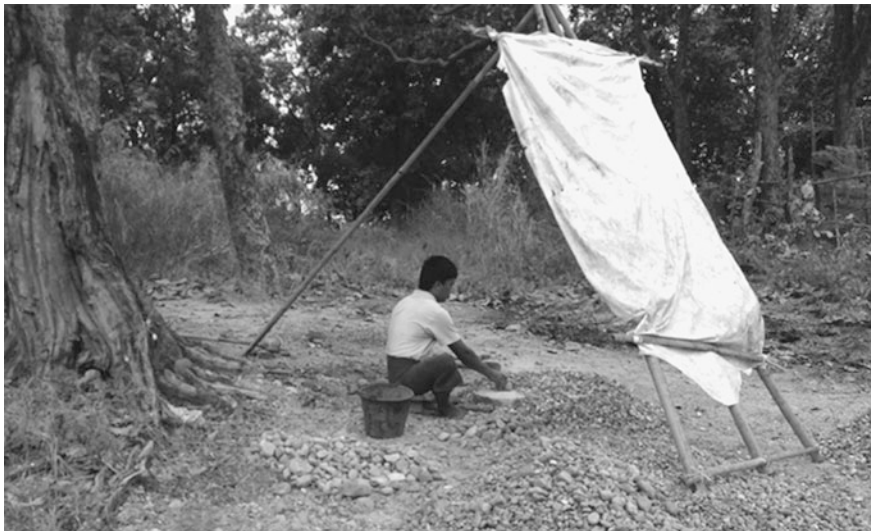
Fig. 8 Handmade construction aggregate from “Potato Stone” (photo by author)
