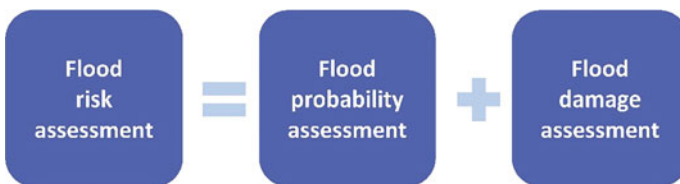
Fig. 1 Coupling models and tools for flood probability assessment and flood damage assessment to assess flood risk (Luther and Schanze 2009)
