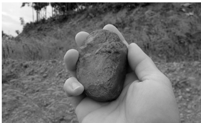
Fig. 7 “Potato Stone” for producing construction aggregate (photo by author)
