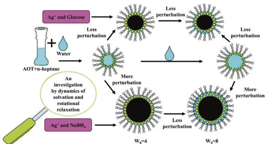
**Fig. 2** Effect of the different reducing agents (glucose and sodium tetrahydroboride) on the size of silver nanoparticle synthesized in bis(2-ethylhexyl) sulfosuccinate sodium salt/n-heptane system. Sodium tetrahydroboride thus produces bigger size of silver nanoparticles, which causes more perturbation to reverse micelles. Chaurasia and Hebbar, Chap. 5
