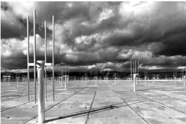
**Fig. 12.** *GRAVES Space Surveillance System: receiving antennas (source: ONERA).*
