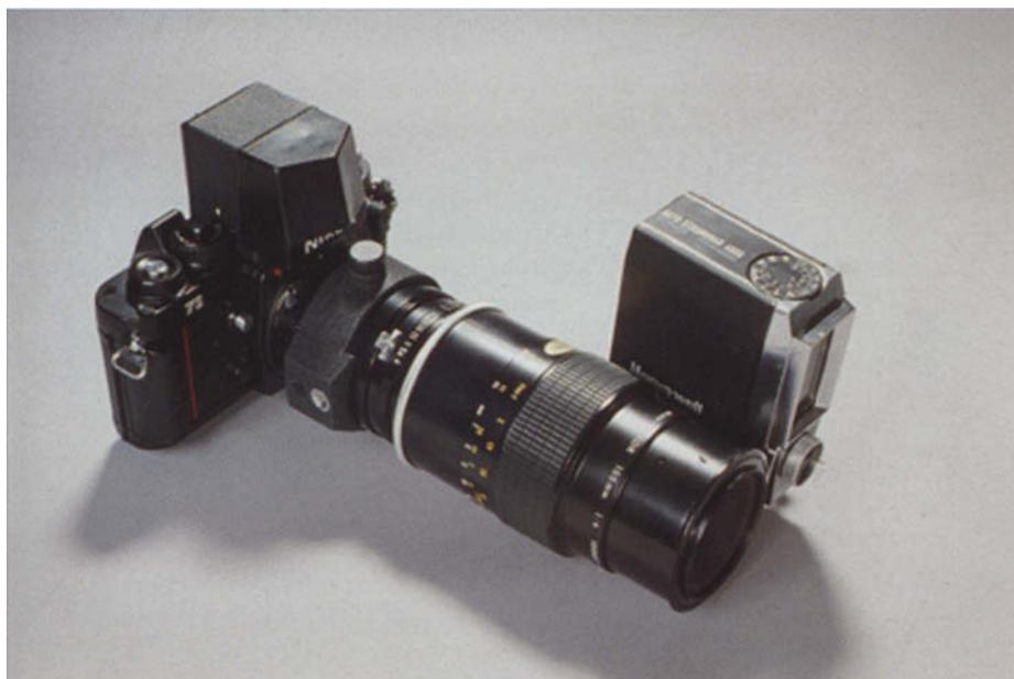
**FIGURE P-2.** Nikon camera with 100-mm macro lens attached for close-up views. A sports viewer is used, and the position of the light source is at the side of the lens.
