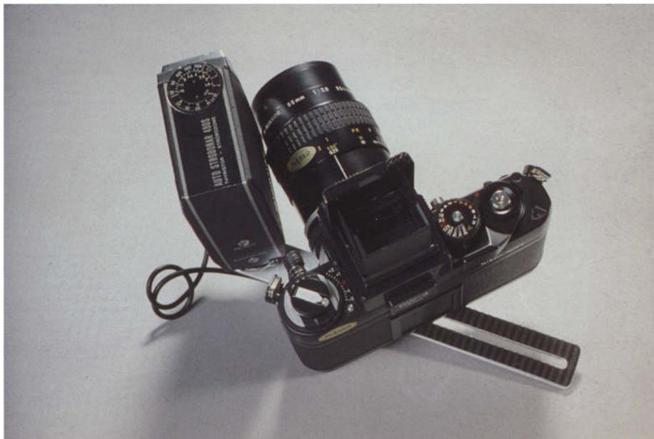
**FIGURE P-1.** Nikon camera viewer from above. A 5-mm macro lens is attached, and the light source is positioned to the side of the lens. A waist-level viewer is attached for taking pictures from the head of the operating table.
