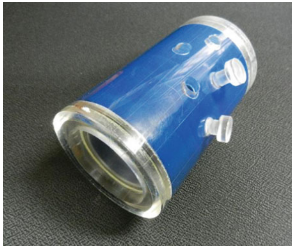
Fig. A.5 Cylindrical test section made of ultrasonic absorbing material (AptFlex; see Table A.6)
