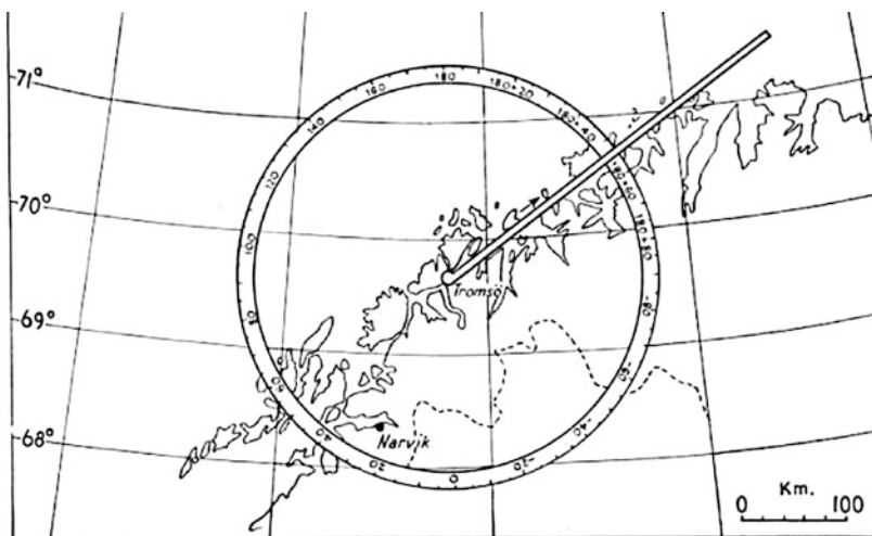
Fig. B.7 Illustration of graphical method used by Størmer to specify the geographical locations and orientations of auroral forms (Størmer, 1955, p. 63)
