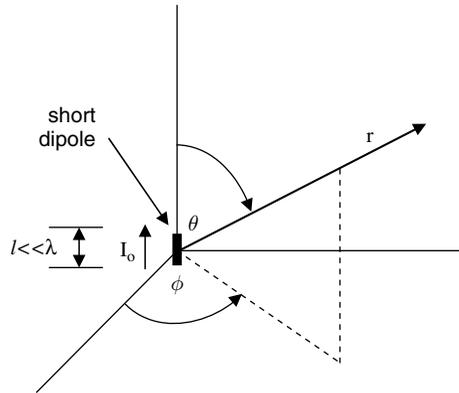
and is so short that there is no distribution of current along its length at any time, then the complete set of fields generated about the short dipole is
