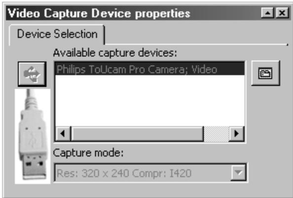
**Fig. B.11.** Configuration page of the *Video Capture Device* macro in processing mode. In this mode only the “Show device properties” button is enabled to display and change the device dependent property dialog.
