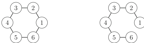
Fig. A.3 Left a simple cycle. Right a simple path yielded by F = \{\{1, 6\}\} .
