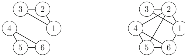
Fig. A.1 Left the graph is not connected, as the cutset defined by \{1, 2, 3\} is nontrivial and empty. Right a connected graph.
