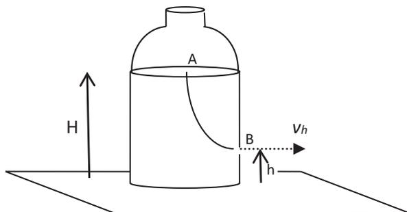
**Fig. E.1** Application of Bernoulli's theorem at two points on a streamline for the flow of water within the bottle
