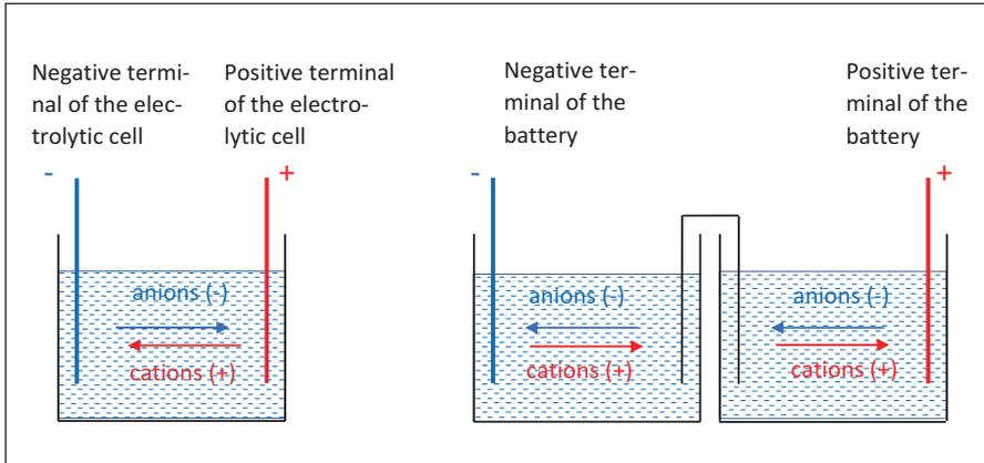
**Fig. F.1** The migration of ions in an electrolytic cell is often explained by the fact that the (positively charged) cations are attracted by the negative electrode of the electrolytic cell and that the (negatively charged) anions are attracted by the positive electrode of the electrolytic cell. It is intriguing to see that the migration of ions in a battery is in the opposite direction
