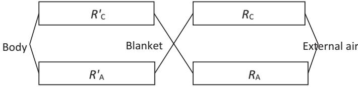
**Fig. H.2** Electrical analogy for the transfer of energy between a person to be protected and the external environment
