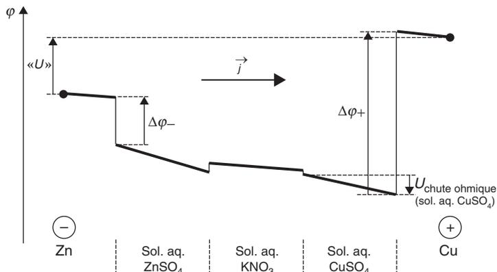
**Fig. F.4** Potential profile in a Daniell electrochemical cell (Lefrou et al. 2012, p. 73).  $U$  is the potential difference between the terminals of the cell, the terms  $\Delta\phi^-$  and  $\Delta\phi^+$  represent the potential drops between each electrode and the liquid.  $\vec{j}$  is the current density
