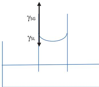
The force that lifts the liquid is  $\gamma_{SG} - \gamma_{SL}$
