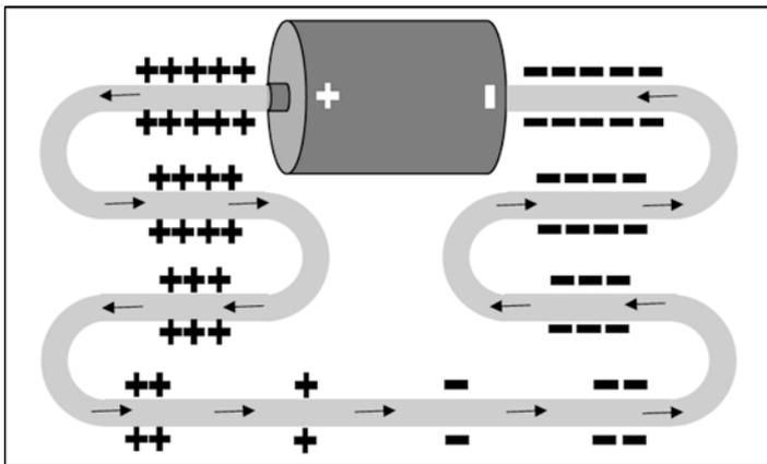
**Fig. F.2** (repeat of Fig. 2.10): Charge distribution in a simple electric circuit in a quasi-stationary regime. Surface charges are represented at different points of the circuit so that the charge gradient and the resulting field are explicit. See in particular Chabay and Sherwood (2006). Not shown here, the charges located on the curved parts of the circuit are essential to explain that electrons follow (on average) the wires
