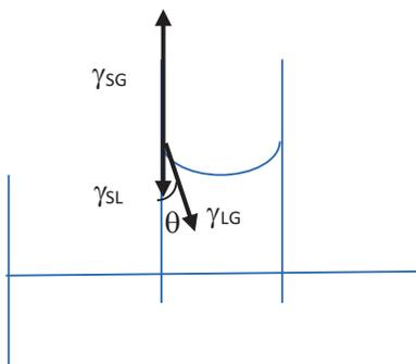
**Fig. G.2** A common explanation of the capillary rise (notations as in the previous figure)
