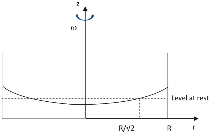
**Fig. G.4** Dynamic equilibrium for a rotating fluid in a cylindrical centrifuge of radius  $R$  at constant rotation velocity  $\omega$
