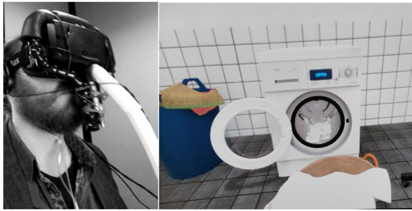
Fig. 1 A view of the olfactometer connected to the Oculus Rift (left), and what a participant sees from within the VR environment (right)
