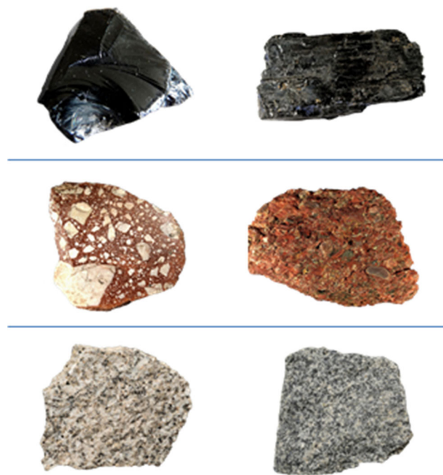
Fig. 2 Representative tokens of selected pairs of subtypes with high within-pair similarity and low between-pair similarity. Top panel: obsidian ( left ) versus anthracite ( right ); middle panel: breccia ( left ) versus conglomerate ( right ); bottom panel: granite ( left ) versus diorite ( right )
