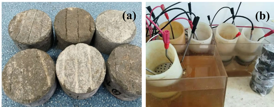
Fig. 3 a Coring diagram of 3DPC specimen and b chloride ion migration test
