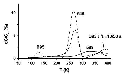
**Figure 1.** DLTS spectra with electrical injection measured for samples 598, 646 and B95. Measurement conditions: reverse bias of -0.5V, forward bias of 1V (2 s duration),  $t_1/t_2$ =100/1000 ms (for sample B95 we also show the high temperature portion of the spectrum measured with  $t_1/t_2$ =10/50 s)
