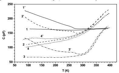
**Figure 3.** C-T curves for various GaN samples measured at 1 kHz when cooling in the dark (1,2,3,4) and after illumination with the deuterium UV lamp at 85K (1',2',3',4'). Curves 1,1' are for sample 598,2,2' for sample B95,3,3' for sample 646. Also shown are the cooling down and heat-up curves for sample B95 illuminated with UV light and quenched with forward bias pulse of 0.8 V (curves 4,4'; note that only the signal from PPC due to ET4 trap can be seen).
