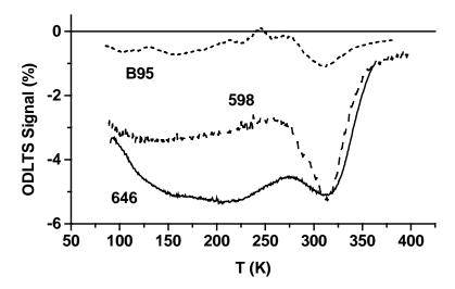
**Figure 2.** ODLTS spectra in samples B95, 598 and 646; measurements were made at -0.5V reverse bias, with a UV deuterium lamp injection pulse 2 s long; the spectra are shown for time windows  $t_1/t_2=100/1000$  ms.
