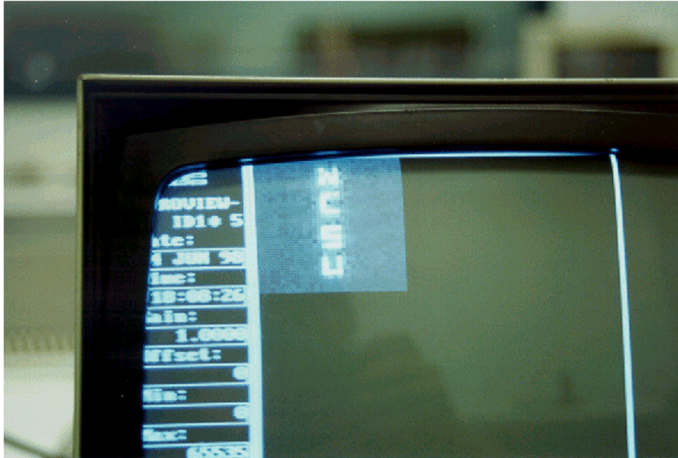
Figure 11. First demonstration of a visible-blind UV image from a III-V nitride-based photodiode array. The image from the FPA was recorded at NVL on July 28, 1999.
