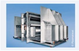
Surfaces of rolled goods with a width of up to 1.5 m can be treated with this low-pressure plasma system.
