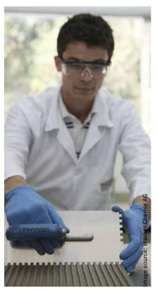
At the Technical Centre of Wacker Química do Brasil, application engineers test products and formulations for the South American market. The expansion focuses mainly on the laboratories for dispersible polymer powders, which are used in drymix mortars for concrete applications, tile adhesives and sealing slurries, for example.
