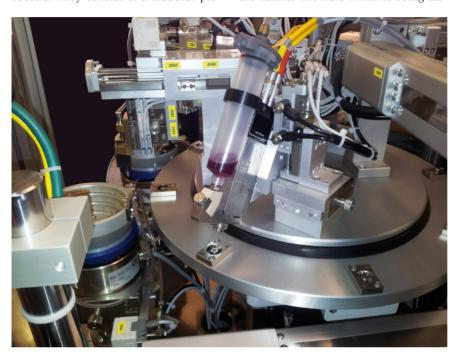
pensed reaches the nozzle at high speed and under high pressure, because the dispensing pressure is significantly higher than the supply pressure. As a speed of more than 1000 cycles per second is possible, the fluid can be applied to the substrate using a non-contact process from a certain distance away.
