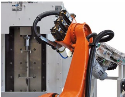
The special gripper system developed for the loading and unloading robot can pick up the cylinder heads in two different positions.
