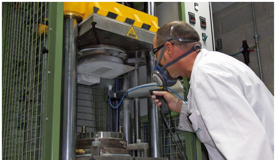
Spraying the powder into the SMC mould. New coatings allow SMC parts to be moulded and coated in one operation.
