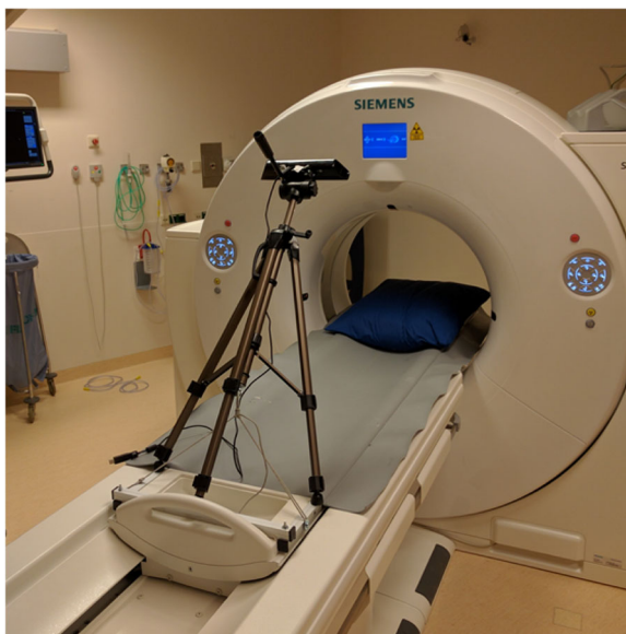
Fig. 1 CT table setup. Setup of the Kinect camera on a CT table, positioned with its field of view into the gantry. The tablet can provide visual biofeedback to patient and operator
