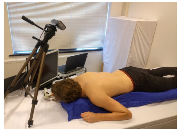
Fig. 2 Experimental setup. Setup of how the Kinect was used in this study. Volunteers could see the visual biofeedback on the additional screen
