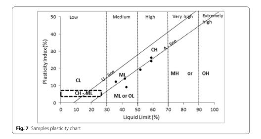
the high LL coupled with high clay content might certify the soils as problematic soils that could be susceptible to landslides [47].
