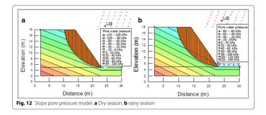
might be imminent since the activating forces would be greater than resisting forces. It is noteworthy to say that the volume of the sliding materials in landslide episodes could be increased with water in and around the slopes. This assertion was evident from the numerical analysis were the sliding mass increased from 67.97 to 71.51 m<sup>3</sup> as water increased within the tailing slope as seen in Fig. 10b, f. This observation is inconsistent with the findings of Maduka et al. [38].
