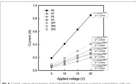
**Fig. 3** Current–voltage characteristics of the CNF/PVDF-HFP composite coated on cotton fabrics with various circuit patterns
