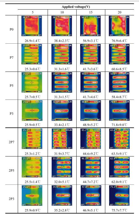
**Fig. 4** IR thermal image of surface temperatures at various applied voltages of the CNF/PVDF-HFP composite coated on cotton fabrics with various circuit patterns
