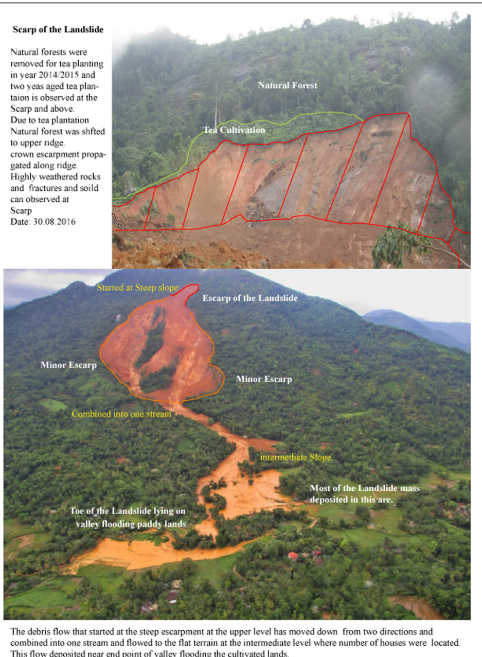
Fig. 2 Figure illustrates escarpment of the landslide, evidence for human intervention in escarpment and above it and difficult translational path of the debris flow
