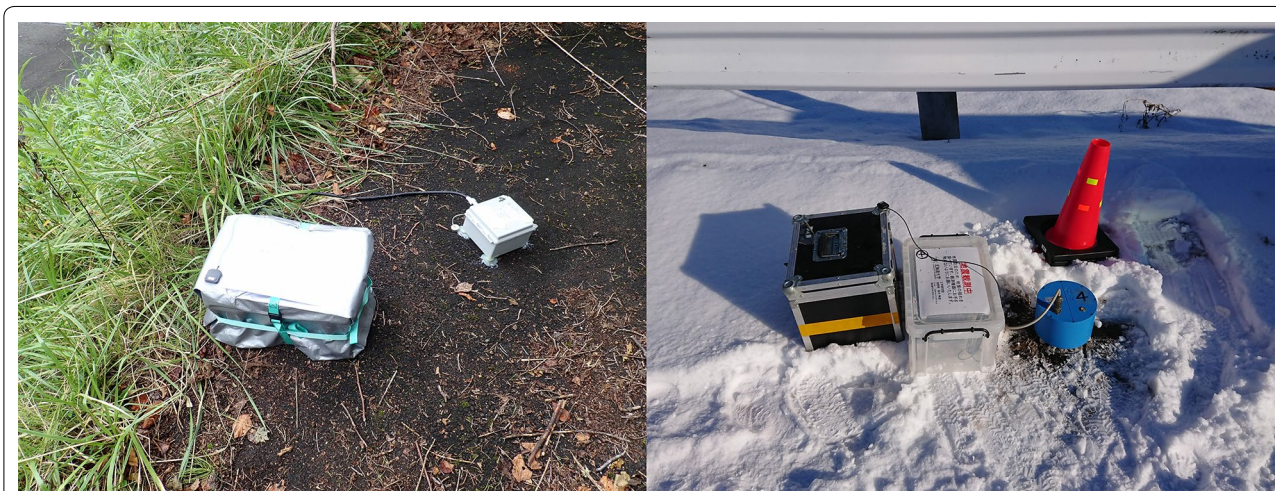
Fig. 6 Photographs of the setting situation. The temporarily strong motion station (left: MKW01). The microtremor observation (right)
