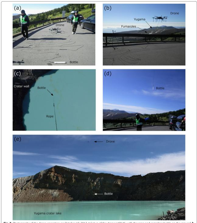
**Fig. 2** Photographs of the drone operation on October 18, 2017. **a** Setup of the drone LAB645, with the rope and sampling bottle on the ground. **b** Taking off with the suspended sampling bottle. **c** Photograph above sampling point B shown in Fig. 1, taken by a camera on the drone. **d** Catching the bottle by hand just before landing. **e** Approach of the drone and sampling bottle to the surface of Yugama crater lake
