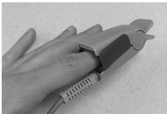
Figure 2 Example of a finger pulse oximeter. This illustration was created for the current article.
