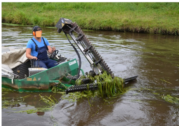
Fig. 2 Boat-mounted cutting device (source: Sandra Roth)
