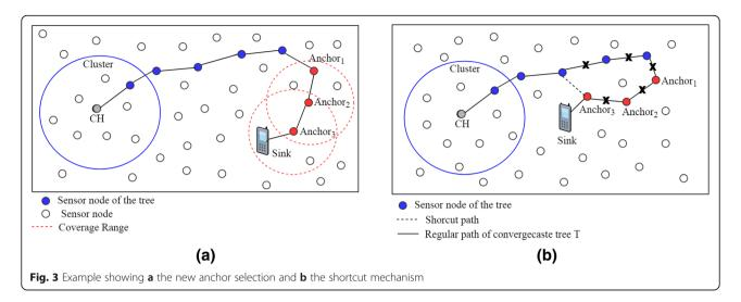
To save energy and to reduce the event-reporting delay, we implement a *shortcut* mechanism. If a node  $N_j$  in T receives beacons from the last anchor, then  $N_j$  stores this anchor as its parent  $N_j$  .tp. Then  $N_j$  sends data directly to the last anchor instead of sending it through the rest of the path. This mechanism is illustrated in Fig. 3b.
