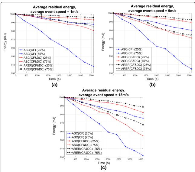
**Fig. 4** Average residual energy of the network with different speeds of the event. **a** Average event speed 1 m/s. **b** Average event speed 9 m/s. **c** Average event speed 18 m/s
