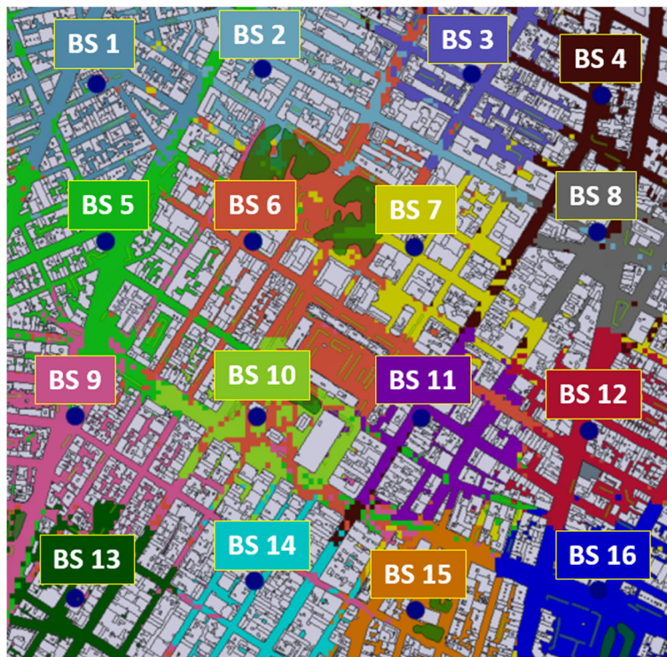
Fig. 4 Massive MIMO BS deployment area. The BSs are depicted by blue dots. The study area is 1.35 km 2 . The different colors in the streets represent the color corresponding to their best serving BS for that area
