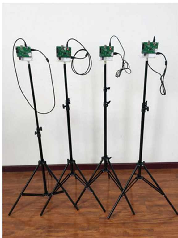
Fig. 7 Base stations. The base stations adopt the STM32103RC chip as the control unit, and each base station has an extra Wi-Fi module called ESP8266, which is used to connect with the server
