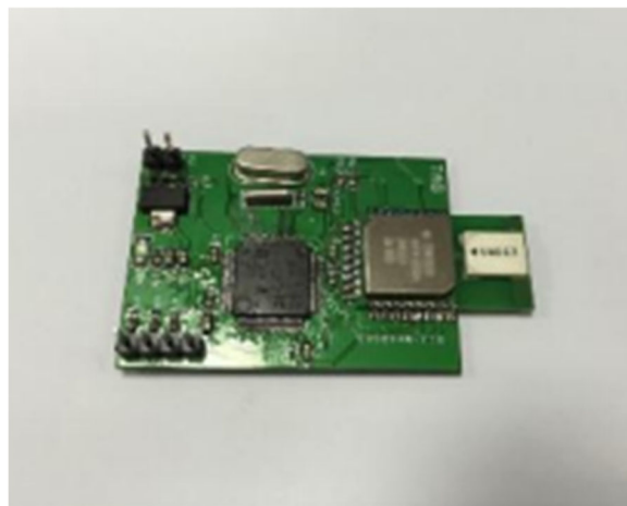
Fig. 6 The tag. The tag adopts the STM32103RC chip as the control unit, and it contains DWM1000 module as the ultra-wideband wireless transceiver
