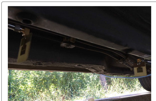
Fig. 2 Transmit and receive antennas beneath the chassis
