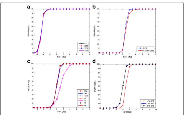
Fig. 7 PSMFRs of radar pulse modulations at different SNR values: (a) Basic IMOPs in CFM family; (b) Basic IMOPs in DFC family; (c) Basic IMOPs in DPC family; and (d) Hybrid IMOPs in the DFC and DPC families
