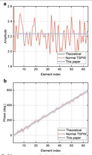
**Fig. 8** The reconstruction results when the weighting circuit is not ideal. **a** and **b** are the amplitude and phase, respectively
