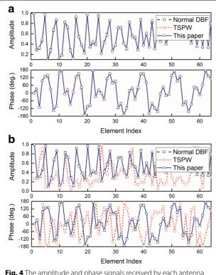
**Fig. 4** The amplitude and phase signals received by each antenna element in the **a** static and **b** moving scenarios, respectively
