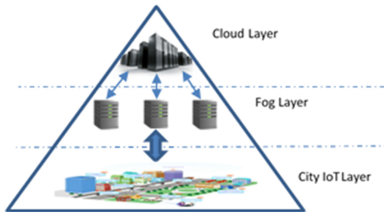
Fig. 1 An Illustration of the integration of IoT, fog computing, and cloud computing to support smart city applications
