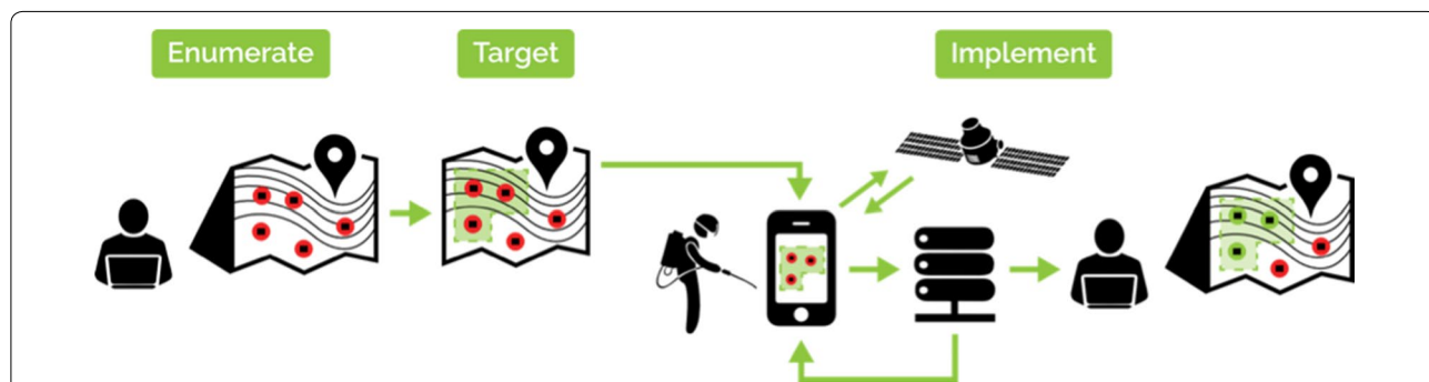
Fig. 1 mSpray consists of enumeration of all structures from satellite maps, selection of households for IRS using a targeting methodology and finally spatial data collection with near real-time reporting/feedback. The figure shows from left to right, Enumerate—computer-based satellite enumeration, target—a map of enumerated structures (red dots) and target areas (green), implement—a tablet-based map to guide users to targeted structures where spatial data is collected, reported to a server and then visualised on intuitive interactive dashboards
