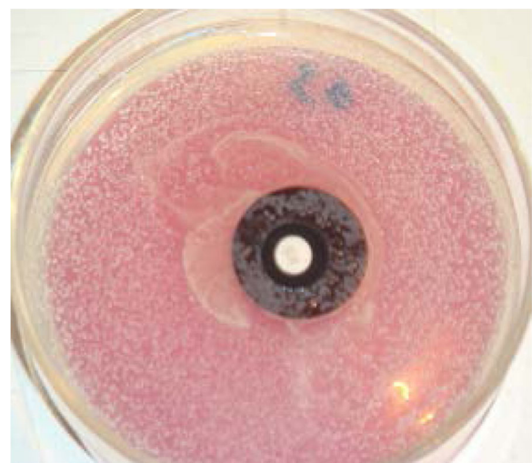
Fig. 3 Shows no zone of inhibition around the black poly carbonate with the biofilm developed on it. Antibiotic disc is placed in the centre
