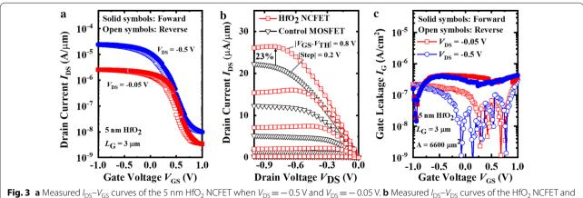
the control MOSFET. **c** Measured  $I_{CS} - V_{CS}$  curves of the 5 nm HfO<sub>2</sub> NCFET when  $V_{DS} = -0.5$  V and  $V_{DS} = -0.5$  V and  $V_{DS} = -0.5$  V.
