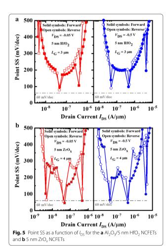
Due to the different ability of scavenging effect for the  ${\rm Al_2O_3/HfO_2}$  and  ${\rm ZrO_x}$  layer, the partical dipoles switching is caused in the  ${\rm Al_2O_3/HfO_2}$  NCFET. Therefore, the
