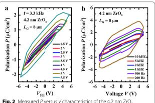
**Fig. 2** Measured *P* versus *V* characteristics of the 4.2 nm  $ZrO_x$  capacitors with **a** different sweeping ranges of *V* and **b** different measurement frequences
