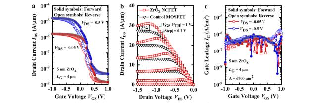
**Fig. 4** a Measured  $I_{DS}-V_{GS}$  curves of the 5 nm  $ZrO_x$  NCFET when  $V_{DS}=-0.5$  V and  $V_{DS}=-0.5$  V. **b** Measured  $I_{DS}-V_{DS}$  curves of the  $ZrO_x$  NCFET and the control MOSFET demonstraing the obvious NDR phenomenon. **c** Measured  $I_G-V_{GS}$  curves of the 5 nm  $ZrO_x$  NCFET when  $V_{DS}=-0.5$  V and  $V_{CS}=-0.05$  V.
