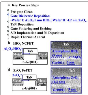
**Fig. 1 a** Key process steps for the fabrication of the  $Al_2O_3/5$  nm  $HfO_2$  NCFETs and 4.2 nm  $ZrO_x$  NCFETs. **b** Schematics and **c** HRTEM images of the fabricated  $ZrO_x$  NCFETs. **d** Schematics and **e** HRTEM images of the fabricated  $Al_2O_3/HfO_2$  NCFETs
