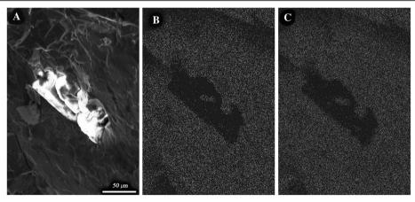
Fig. 2 Diamond crystals of three alloys (a) and distribution maps of aluminum (b) and iron (c)
