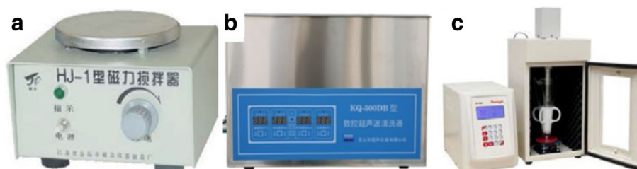
Fig. 1 Images of dispersion instruments. a Magnetic stirrer. b Ultrasonic bath. c Probe
