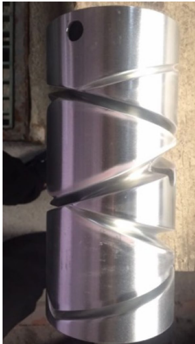
Figure 10 Groove drum component of winder after polishing
