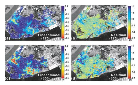
Fig. 10. Subsidence models and residuals for the subsidence during the ENVISAT observation (2004–2005). (a) and (c) Linear model subsidence for 175 and 350 days. (b) The residual map between the 175-day ENVISAT observation (mean of Figs. 8(a) and 8(c)) and the model. (d) The residual map between the 350-day ENVISAT observation (mean of Fig. 8(b) and the scaled Fig. 8(d); see the text) and the model.
