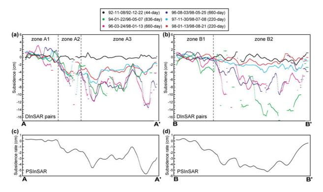
Fig. 4. (a) Subsidence profiles in some typical JERS-1 interferograms along the line A–A' described in Fig. 3(a). Zone 'A1' represents stable area and zones 'A2' and 'A3' represent subsiding area with a different temporal evolution. (b) Subsidence profiles along the line B–B'. (c) and (d) Profiles of the mean subsidence velocity estimated from PSInSAR (see Fig. 6) along the line A–A' and B–B'.
