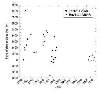
Fig. 2. JERS-1 SAR and ENVISAT ASAR image sets of Mokpo City. The dots and a circle represent the JERS-1 images, and the triangles denote the ENVISAT images with their acquisition dates and relative perpendicular baselines with respect to the first data of each satellite. A circle represents the selected master data in the PSInSAR analysis of the JERS-1 data.
