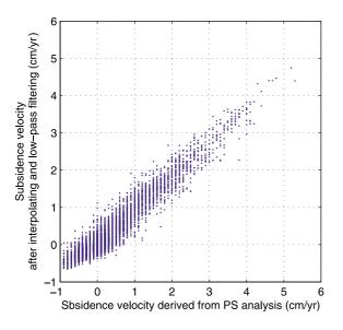
Fig. 7. Scatter plot of subsidence velocity directly estimated from PS analysis and after interplolation and spatial low-pass filtering. The mean and standard deviation of the difference between two velocities is 0.0 and 0.21 cm/yr.
