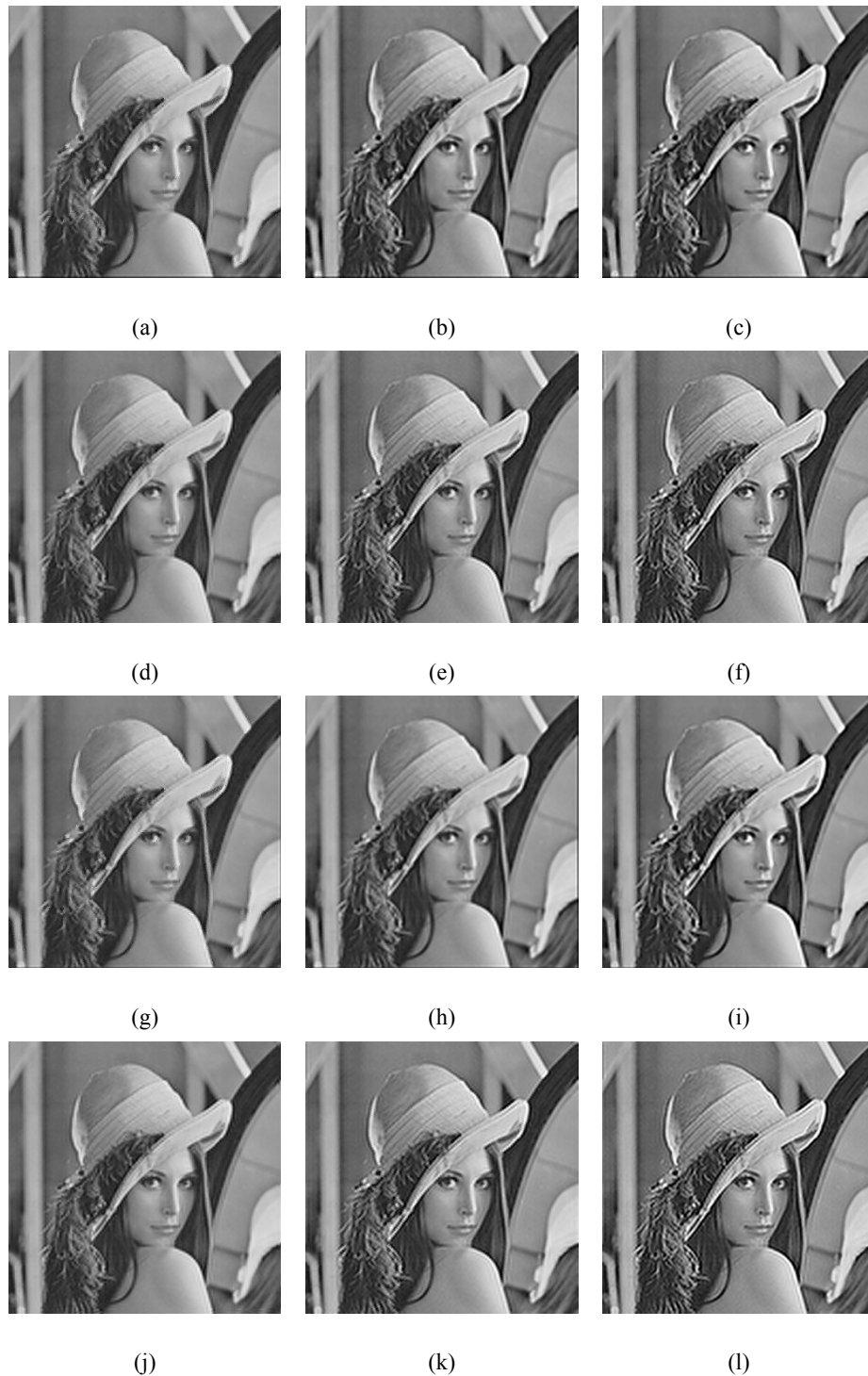
Figure 16 HR image reconstructed by the previously reported methods and the proposed method from the LR images obtained by the Haar and Daubechies filters (Test image "Lena"). HR image reconstructed from the LR image obtained by using the Haar filter by (a) reference [11] (SSIM index: 0.7941), (b) reference [27] (SSIM index: 0.8235), (c) reference [8] (SSIM index: 0.8159), (d) reference [12] (SSIM index: 0.8428), (e) reference [28] (SSIM index: 0.8337), and (f) the proposed method (SSIM index: 0.8542). HR image reconstructed from the LR image obtained by using the Daubechies filter by (g) reference [11] (SSIM index: 0.7950), (h) reference [27] (SSIM index: 0.8455), (i) reference [8] (SSIM index: 0.8148), (j) reference [12] (SSIM index: 0.8458), (k) reference [28] (SSIM index: 0.8320), and (l) the proposed method (SSIM index: 0.8508).
