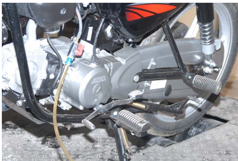
Figure 1 Motorbike mounted on roller test bench.
