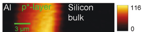
Figure 6 Intensity of the defect luminescence at 1,250 nm in the BSF. The intensity is clearly increased at the right side of the BSF, which indicates a higher defect density here. This could cause the low lifetimes at the interface between BSF and silicon bulk.
