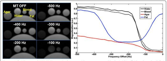
Figure 1 Left: MT-prepared VIPR SPGR scans in phantoms with water, 4% agar, blood-mimicking fluid, and canola oil (fat) demonstrate signal saturations at various MT offset frequencies. Right: Signal calculations over a range of frequencies show maximum fat suppression near its peak at 1.5T.
