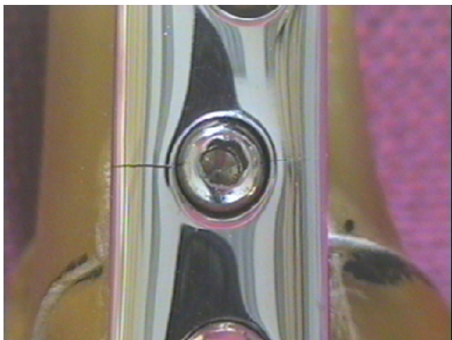
Figure 9 Photograph demonstrating a fracture through a screw hole with a screw in-situ.
