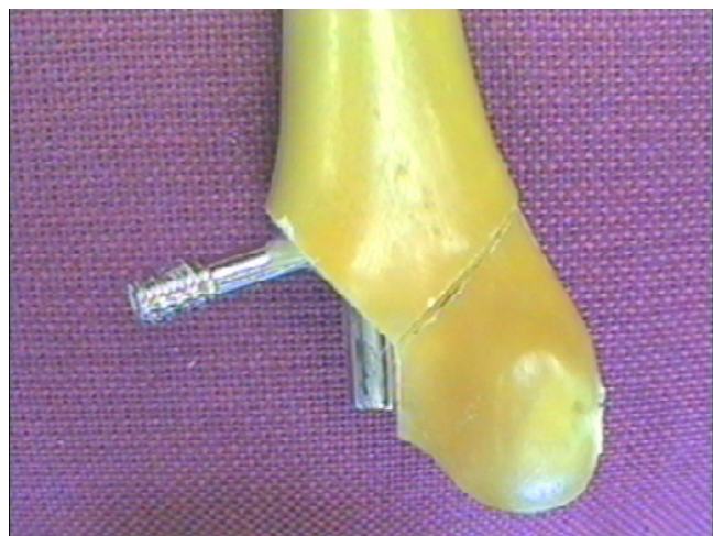
Figure 7 Photograph demonstrating a bent lateral locking screw with nail (Specimen 3).
