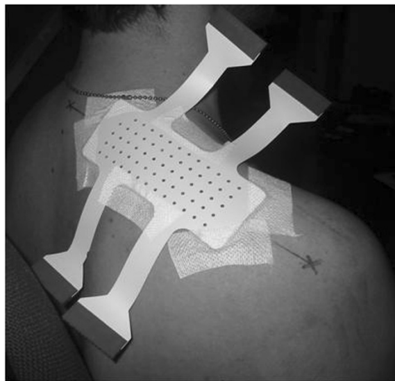
Figure 1 Recording of upper trapezius single-differential signals. Example of the 64 contact electrode matrix applied to the upper trapezius muscle.
