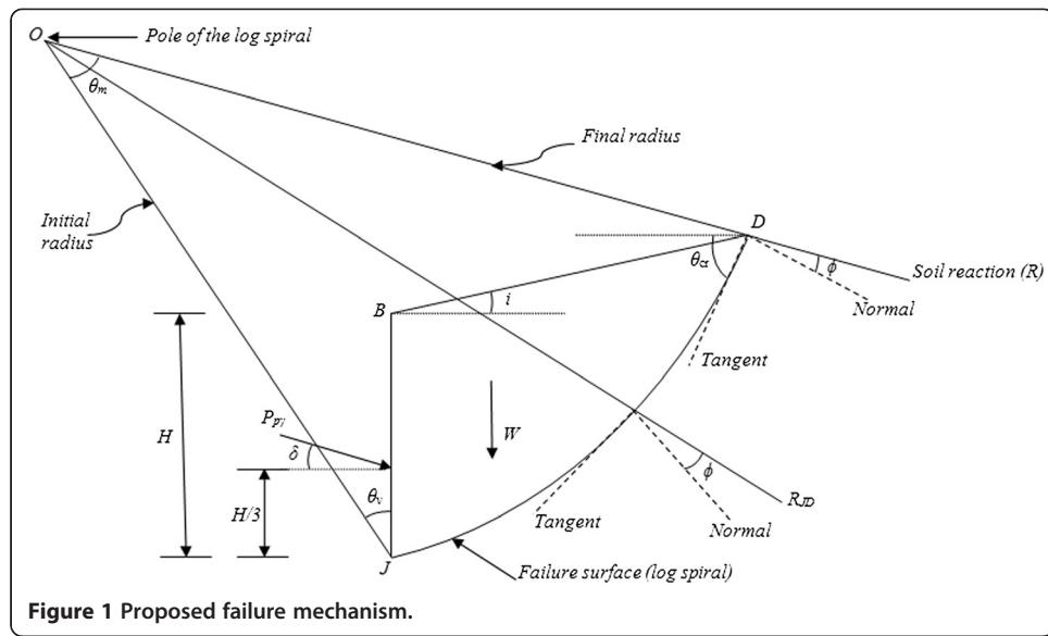
**Figure 1** Proposed failure mechanism.
