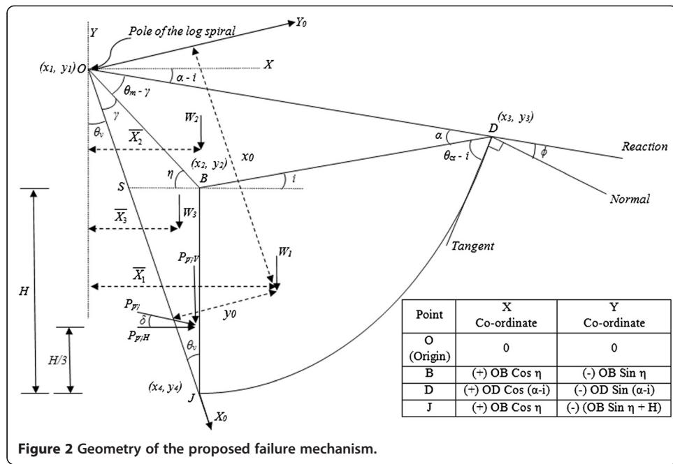
**Figure 2** Geometry of the proposed failure mechanism.
