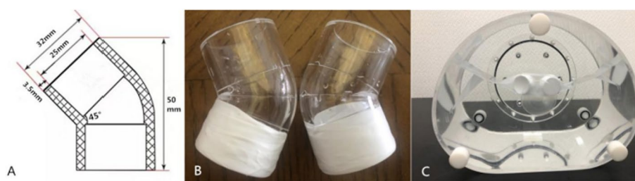
Fig. 1 Thyroid model. A Single elbow size, B bilateral lobe model, C specific T/B thyroid model
